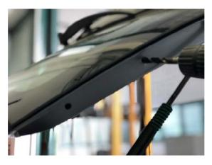
NOW USE A RIVETER TO PUT THE M6 RIVETS INTO THE DRILLED HOLES AND TO BLOCK THEM TIGHT.
