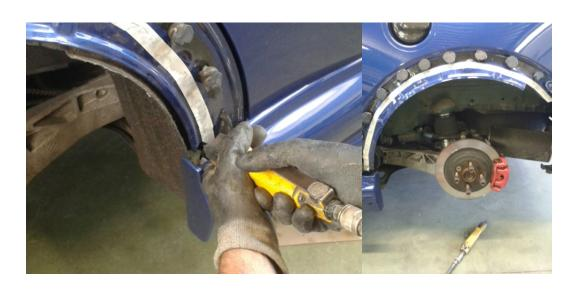
DON'T FORGET TO SEAL THE CUT METAL WITH SOME SEALER OR PROTECTING PAINT TO AVOID RUST UNDER THERE.
