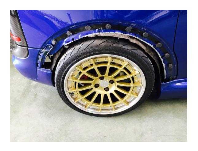
AS YOU CAN SEE FROM THE PICTURES, YOU NEED TO CUT METAL 0,5 CM OFF THE HOLES FOR STANDARD WHEEL ARCHES.
