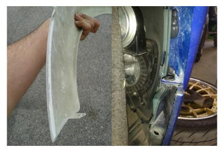
FIBERGLASS ARCHES ARE MORE RIGID THAN PLASTIC BUMPERS: THAT'S WHY PARTICULAR ATTENTION HAS TO BE PUT ON BORDING AND SEALING THE CORNER OF WIDE ARCHES WHICH LINK WITH THE BUMPERS CORNERS.
