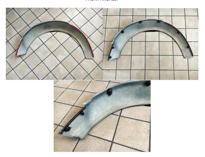
PLACE DOUBLE SIDED TAPE 1 MM BELOW THE EDGE OF THE PERIMETER OF THE ARCHES, ONLY WHERE YOU SEE THE TRACK FOR BONDING (ON REAR ARCHES YOU WILL PUT TAPE ON THE WHOLE PERIMETER).
